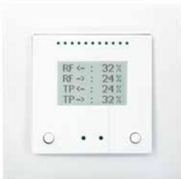
**ELSNER** The KNX RF LC-TP media coupler supplements existing or newly installed KNX TP systems with the KNX RF KNX RF standard. The media coupler is the interface between wire and radio and enables bidirectional data exchange between wired (KNX TP) and wireless (KNX RF) KNX devices. It forwards the telegrams received via radio or wire and displays addressing, bus load and telegram flow between source and destination addresses. Due to its size of 55 x 55 mm, it fits in standard frames.
